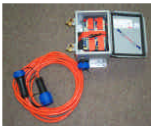
Figure 12 : Battery power enclosure with cabling
