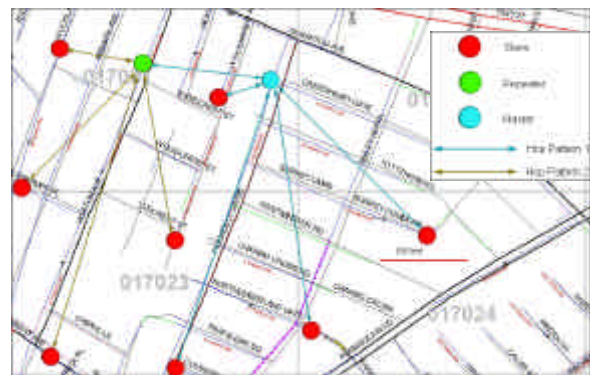
Figure 14 : Wireless network topology example
